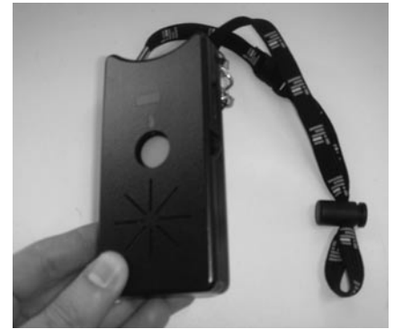
Fig. 1 Portable sensory platforms (Social Badges) used to collect personal communications data
